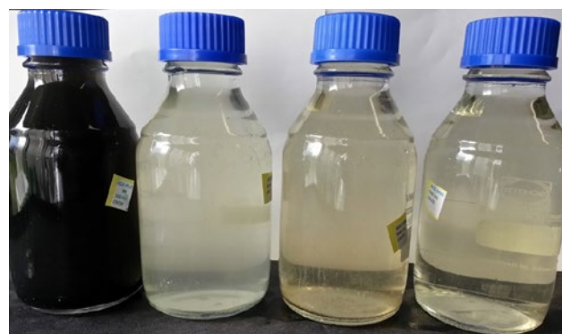
Figure 2 A: High strength wastewater influent (extreme left) and finally treated effluents collected from selected DWWT-technologies.
